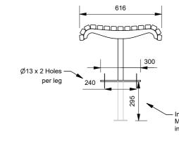
Inground Option Minimum in-ground installation depth
