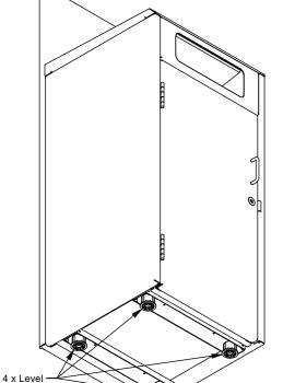
**1.** Place bin surround at intended position on concrete surface. (*Recommended min. slab depth: 100mm.* Ensure feet no closer to the edge of slab than 100mm)
