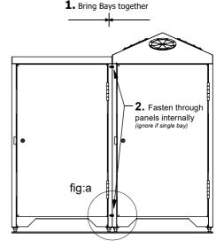
**3.** Join as many bays together as needed. (ignore if single bay) \*Bay openings can be configured in any order and can face the front or the back
