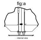
**5.** Using Leveling Strap mounting holes as a template, drill ground surface to suit chosen ground anchors then fit ground anchors.
