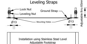
Fixing minimum 100mm from edge of slab
