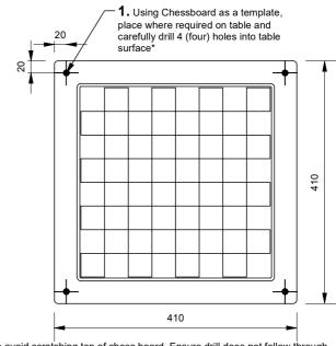
\*To avoid scratching top of chess board. Ensure drill does not follow through after hole is complete.
